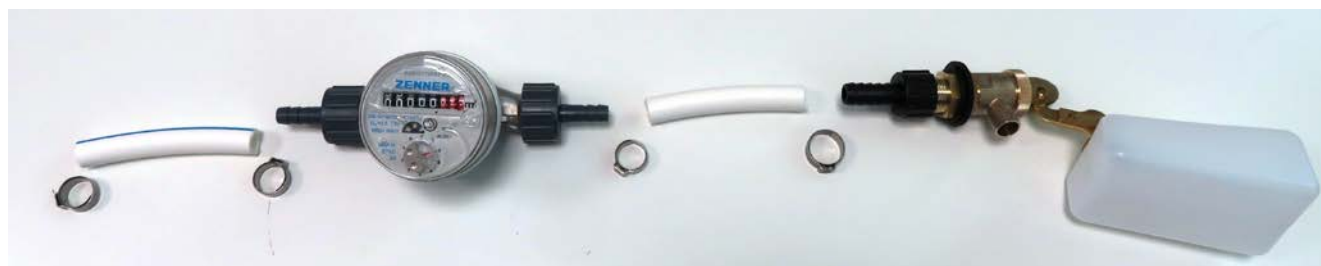
Figure 8: All parts that come with set 2 including water meter (left) and float valve for the FWT (right) and how to connect
