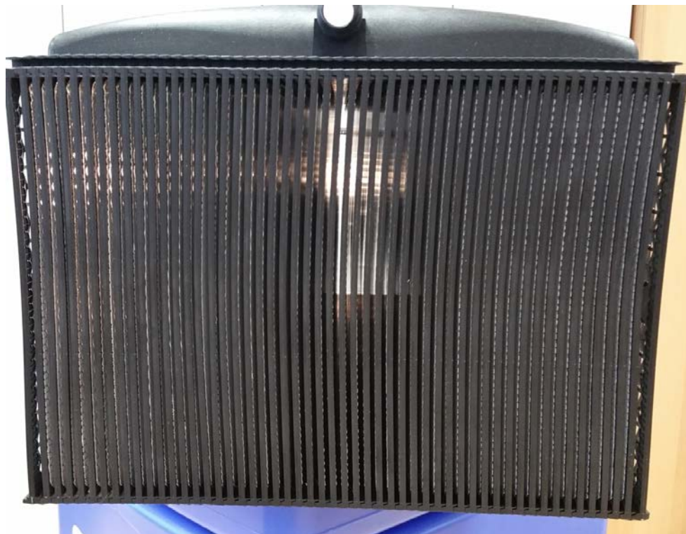
Figure 18: membrane module – look through the slits between the plates
