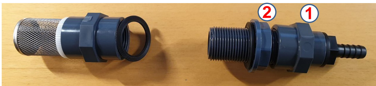
Figure 6: RWT connector parts of set1 (top: ¾" version, down: 1" version) ready for mounting in the RWT
